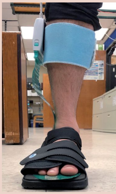
Fig 2. Plantar pressure measurement using F-Scan in-shoe measuring system placed in a standard DARCO surgical shoe
